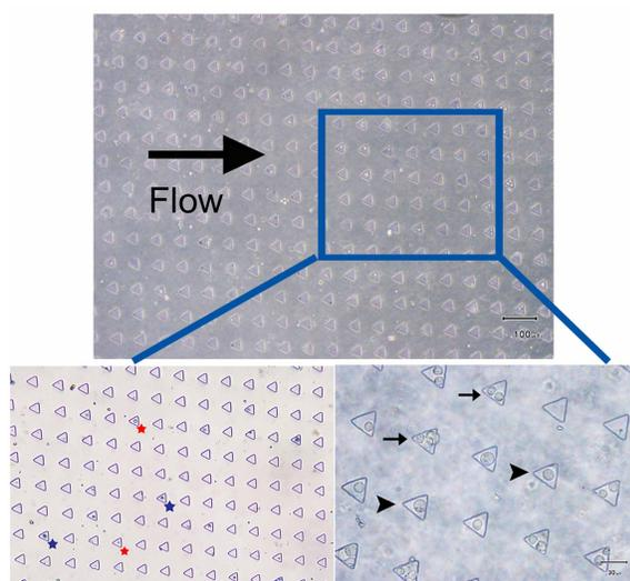
**Fig. 2** Left, Trypan blue staining of trapped cells at 48 h: positive dead cells (Blue stars) and negative living cells (Red stars), 200 $\times$ ; Right, cell trapped in triangular microwells in conventional culture media: single cell (arrowheads) and multiple cells (arrow).
