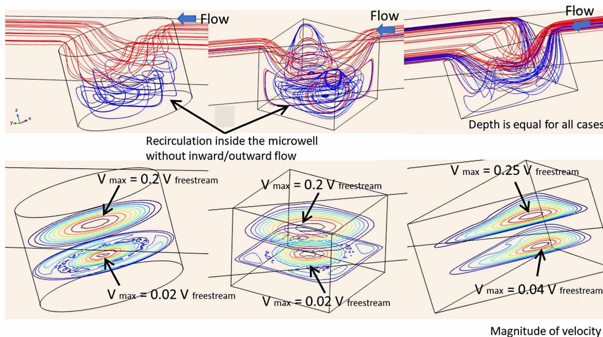
Fig. S1 Streamline and velocity contours for circular, square and triangular microwells of comparable sizes.
