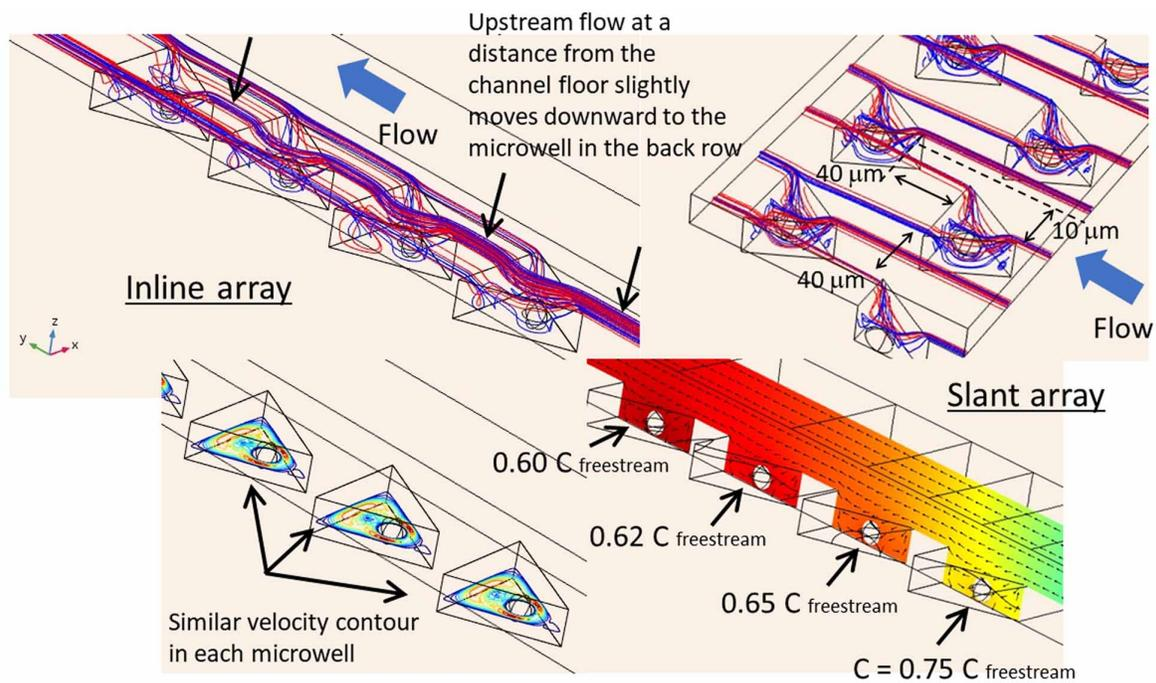
Fig. S3 Schematic pictures of the microfluidic chip comparing inline and slant arrays.
