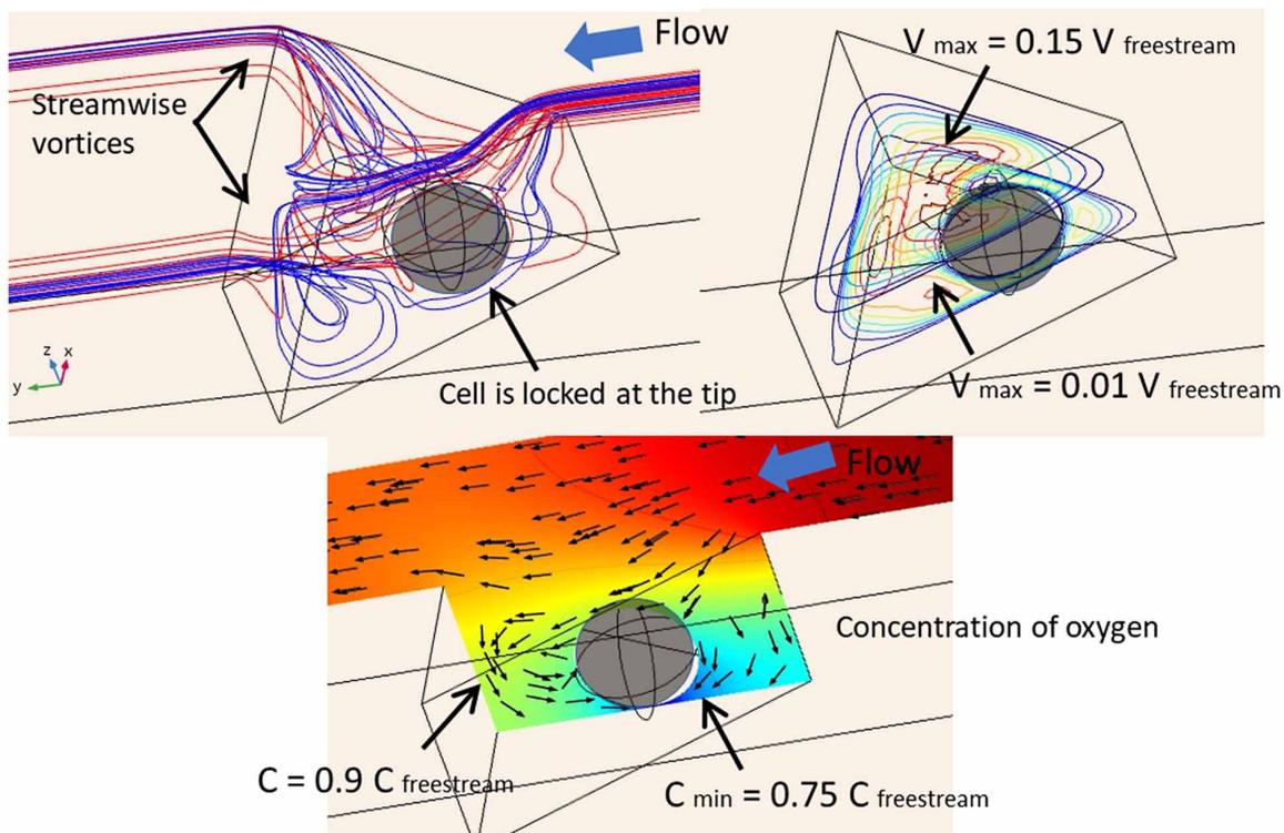
Fig. S2 Streamline, velocity, and oxygen contour inside a triangular microwell occupied by a single cell.
