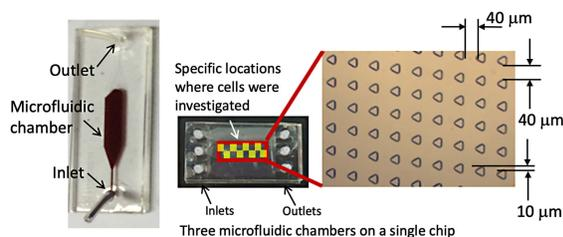
**Fig. 1** A PDMS microfluidic device with an array of triangular microwells placed on a bottom surface.
