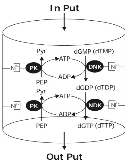
**Fig 4.** Diagram of the strategy of enzymatic synthesis of deoxyribonucleoside triphosphate by immobilization of polyhistidine tagged enzymes on Ni<sup>2+</sup>-NTA agarose. The abbreviations used are DNK for T<sub>4</sub> deoxyribonucleotide kinase, NDK for *E. coli* nucleoside diphosphate kinase, PK for pyruvate kinase, PEP for phosphoenolpyruvate, and Pyr for pyruvate. In this diagram, all three polyhistidine tagged enzymes are immobilized onto the Ni<sup>2+</sup>-NTA agarose in a column.
