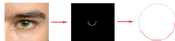
Fig. 6 An example of some process for fitting a circle to data points extracted from the image.
