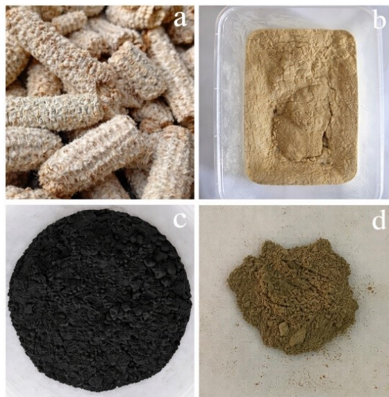
Fig. 1 Preparation of composite: (a) dried CC, (b) CC powder after crushing and sieving to 200 mesh, (c) CCC, and (d) GO/CS/ZnO.
