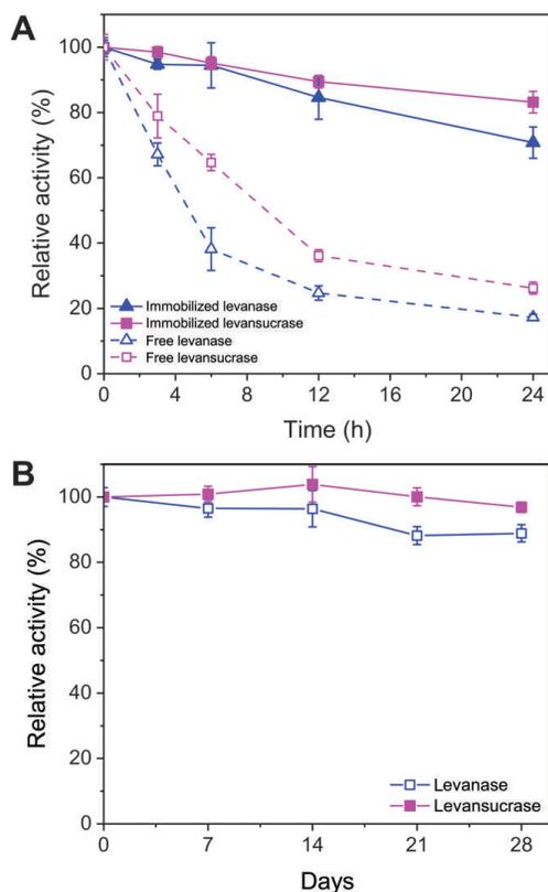
**Fig. 6** Stability of free and immobilized enzymes. (A), Operational stability of enzymes examined at 30 °C, pH 5.0; (B), storage stability of immobilized enzymes stored at 4 °C for 28 days.
