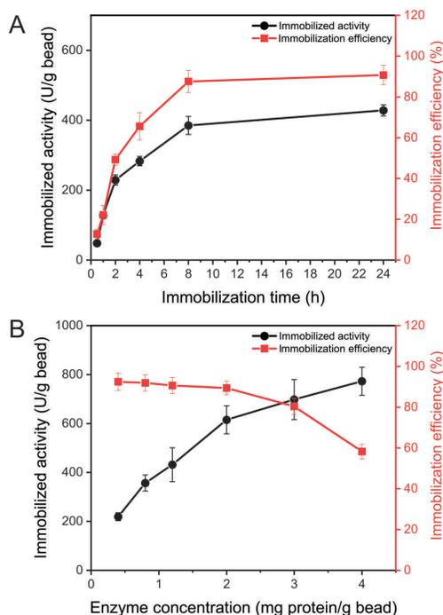
**Fig. 3** Effects of immobilization time, (A); and protein concentration, (B); on immobilization efficiency and immobilized activity of co-immobilized enzymes.
