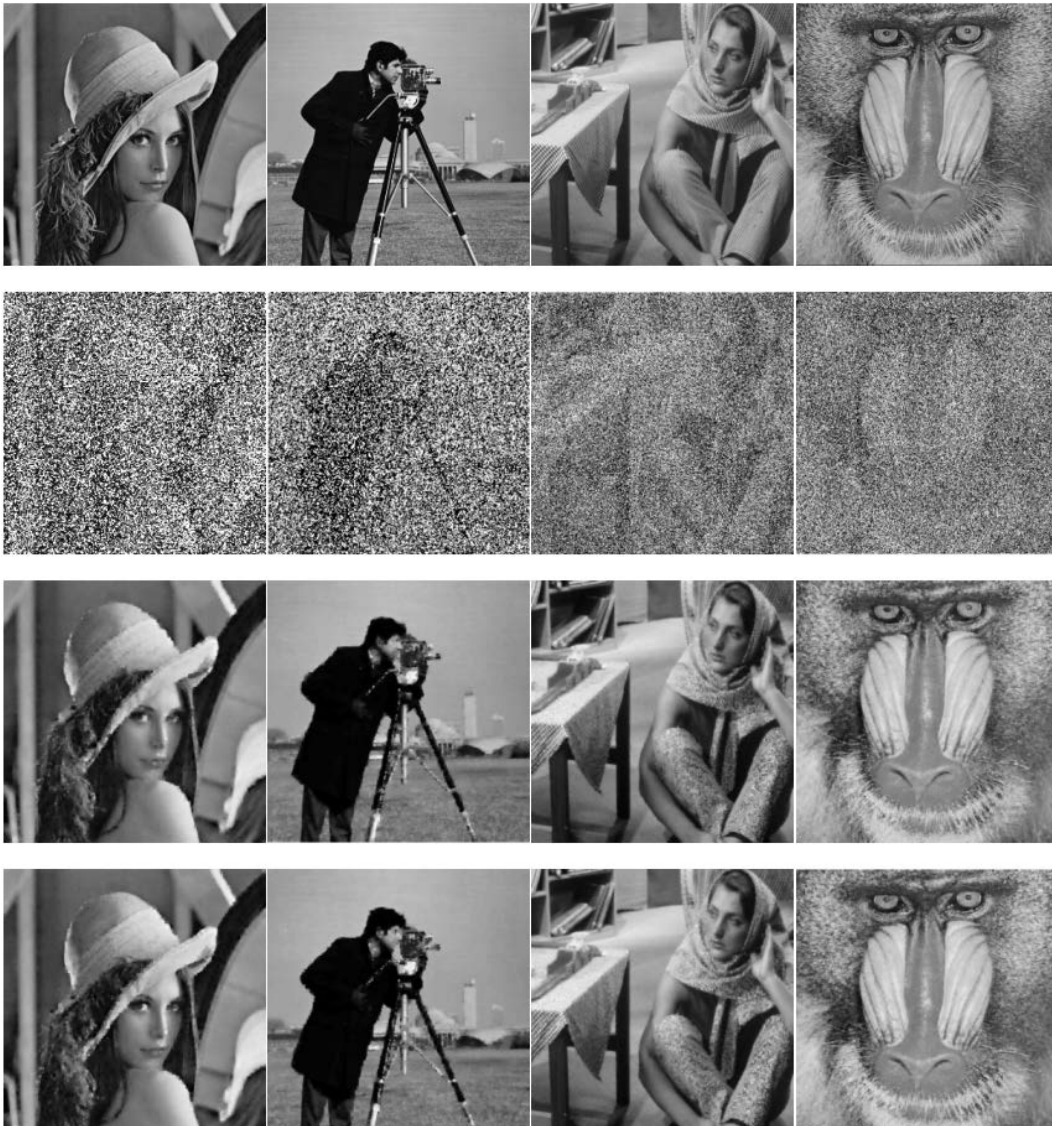
Fig. 2 From top to bottom: original images, noisy images with 0.7 the salt-and-pepper noise, the restorations obtained by minimizing \mathcal{F}_\alpha with TPRP method and Algorithm 1, respectively.
